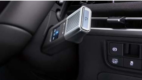
Column-type Shift by Wire (SBW)
